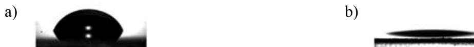
Fig.2: Effect of adding 7% Tween 20 on the contact angle, (a) Water droplet(70°) (b) Water droplet and 7% tween 20 (17°)
